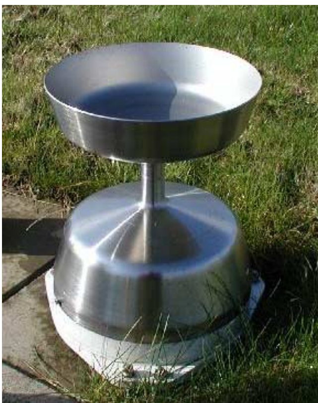
Figure 1 FSS500 Series Raingauge in Situ
