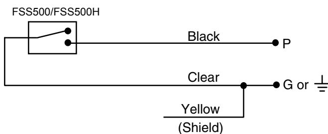
Figure 6 Wiring Diagram for FSS500/FSS500H
