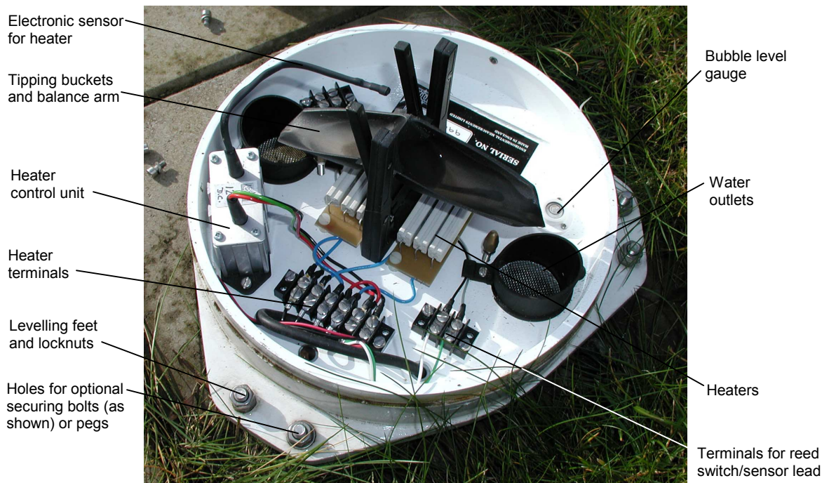
Figure 4 Internal View of FSS500H (Heated Version)
